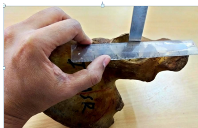
Figure 1: Measurement of depth of acetabulum by vernier calliper using thin acrylic scale
